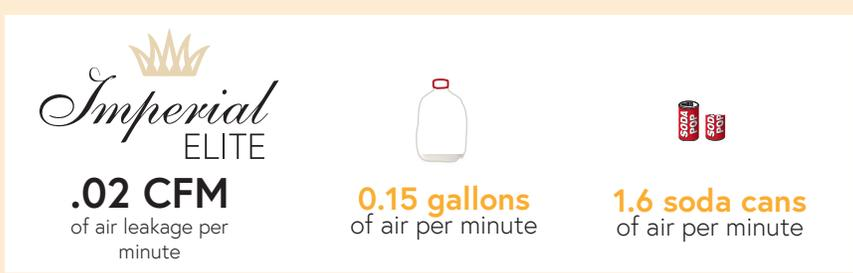
\*INDUSTRY STANDARD: The Fenestration and Glazing Industry Alliance (FGIA) set the industry standard for maximum allowable air infiltration at 0.30 CFM (cubic feet per minute) during a 25 MPH wind. This is equal to 2.25 gallons or 24 soda cans of air leaking through the window every minute!
